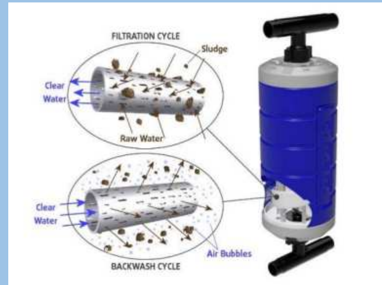
Periodic backwashing with treated water and air scouring
